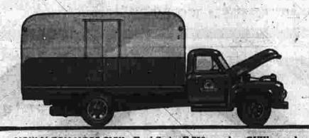
NOW % TON MORE GVW-Ford Series F-750 now has GVW upped to 21,000 lbs. when equipped with heavy-duty rear springs. 152-h.p. Short Stroke V-8 engine. Power Steering available at low extra cost.
